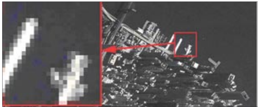
Figure 2. A grid of pixels form a picture – the sharpness of the picture depends on the pixel's density
