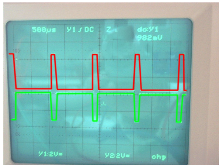
The original signal (green, -3\text{V} ) and after amplification (in red, +5\text{V} )
